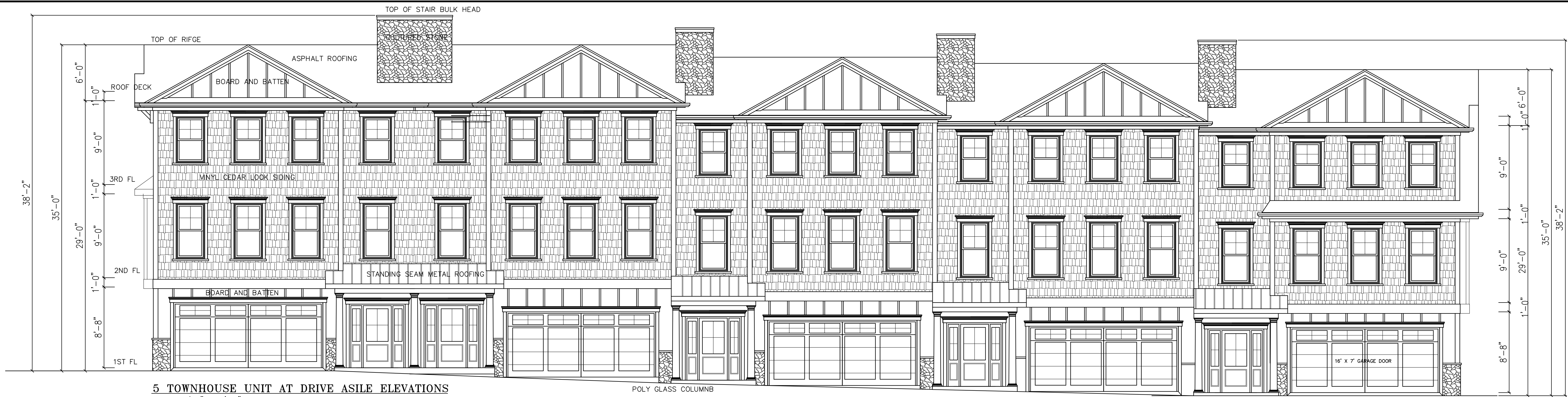
5 TOWNHOUSE UNIT AT DRIVE ASILE ELEVATIONS SCALE 3/16" = 1'-0"
