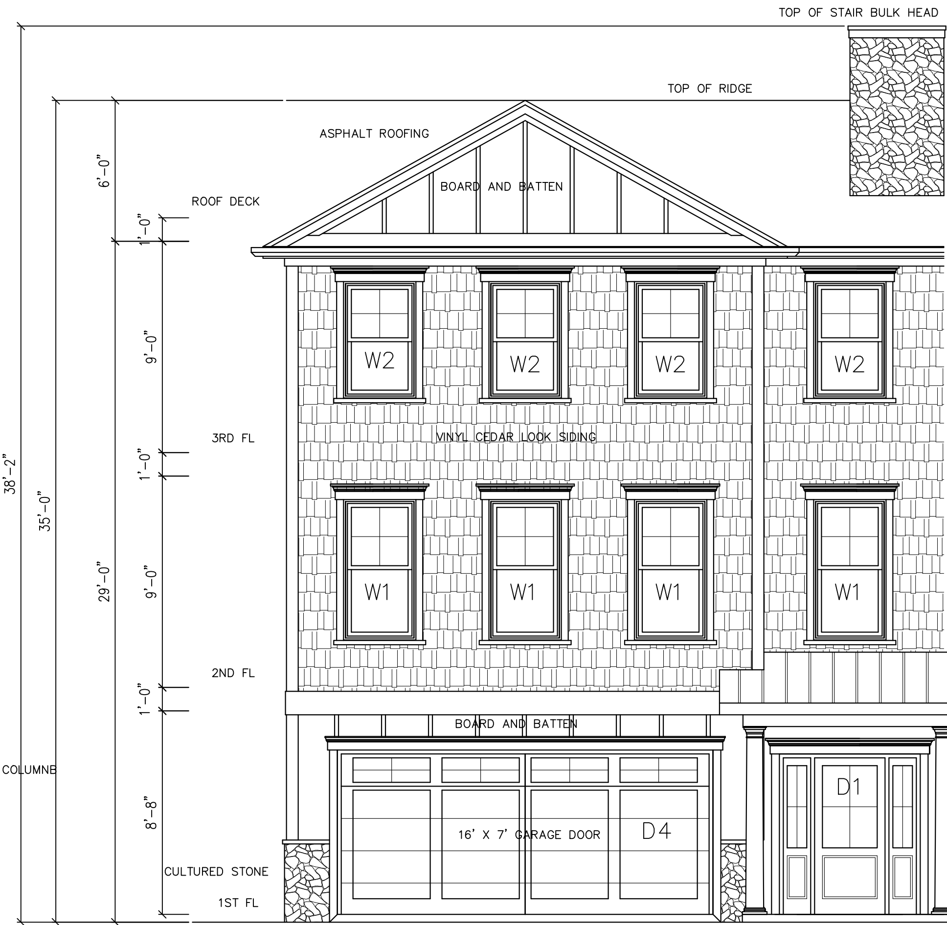
TYPICAL INTERIOR UNIT FRONT ELEVATION SCALE 1/4" = 1'-0"
